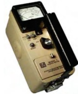
Figure 2. General Purpose Survey Meter
